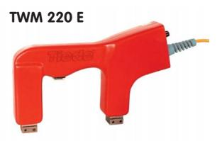
The hand yoke TWM 220 E with replaceable switch and steplessly adjustable regulation is an AC unit and can be directly connected to a 230 V AC supply. Due to the replaceable switch no annoying work interruption will be necessary in case of a damaged switch. By means of the series built-in adjustable regulation device the field strength may be individually adjusted for the different workpieces to be tested.
