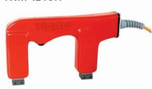
**The AC hand yoke TWM 42 A/N** operates at 42 V supplied from a separate transformer which is connected to a 230 V AC supply. This satisfies the VDE safety regulations so that the TWM 42 A/N can be used for testing in vessels, tubes and closed containers.
