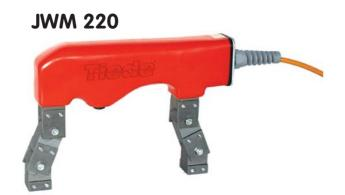
The AC hand yoke JWM 220 is small in size, light in weight, and therefore handy to use. Its magnetization output is adequate to satisfy the majority of test requirements. Articulated pole pieces with twinknuckle adjustment are mounted on the yoke as standard fittings to extend the range of test applications and to ensure the optimum development of the magnetic field within the test piece.
