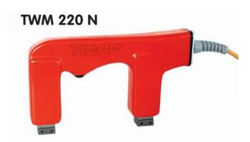
**The TWM 220 N hand yoke** is an AC current instrument that can be directly connected to a 230 V AC supply. In conjunction with adjustable pole pieces it is ideally suited for testing uneven surfaces, tube bends, angle pieces etc.
