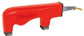
The AC hand yoke BWM 220/12 is of compact construction and is particularly suitable for testing in locations which are confined or difficult of access. The AC hand yoke BWM 220/12 is designed to be connected both to 230 V AC and also, in conjunction with a transformer to 12 V DC.
