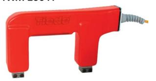
**The TWM 230 A hand yoke** is of similar construction to the TWM-N type, however, the switch on this model can be exchanged when it becomes worn, or faulty. This is done by simply removing the holding screws. We have also introduced a special switching circuit so that the yoke is switched on when the AC current is passing through zero, thereby greatly extending the life of the switch and the yoke.
