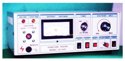
The LH-150T Hipot Tester provides easy table-top dielectric testing of products for domestic or international destinations. Ideal for use in Production Test, R&D Labs, Incoming Inspection or Repair Facilities.
