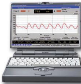
fig. 3: Models ETX and ETPX can be connected to PC for monitoring or downloading stored data (see page C9)
